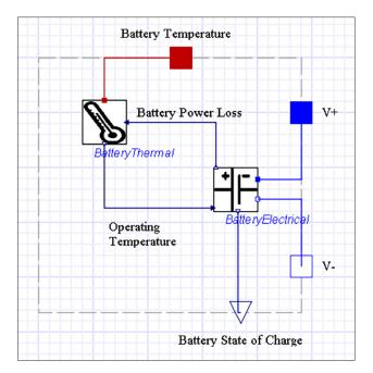
Figure 2. The thermal and electrical characteristics of the battery are easily separated and connected in MapleSim.
