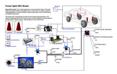
Figure 4. Power-split hybrid-electric vehicle model.
