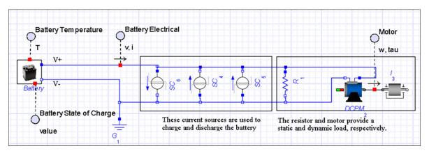
Figure 1. The battery model connected to a variety of loads.
